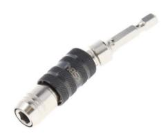
The adjustable head of 30° allows the user to reach difficult accessible spaces. 1/4" hexagonal rod locking in straight position. Quick locking and unlocking. (Single pressure) Powerful magnet.
