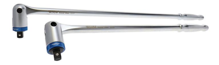
Ratchet wrench with adjustable head of 180°. 3 position ratchet action: right, left or locked. Heavy duty arm to increase working power. Matte chrome satin finish for better corrosion protection.
